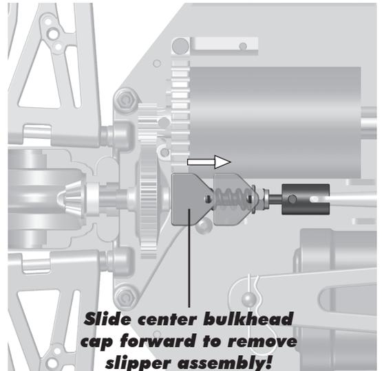
**Slide center bulkhead cap forward to remove slipper assembly!**
